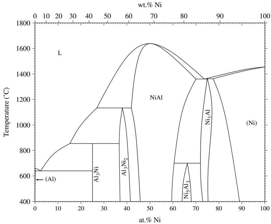
Figure A.9: Binary phase diagram of Ni-Al.
