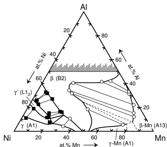
Figure A.10: Ternary phase diagram of Ni-Mn-Al at 850 °C (redrawn from R. Kainuma et al., *J. Alloys Comp.* **269**, 173 (1998)).
