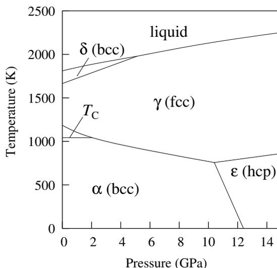
Figure A.11: The pressure-temperature phase diagram of iron.
